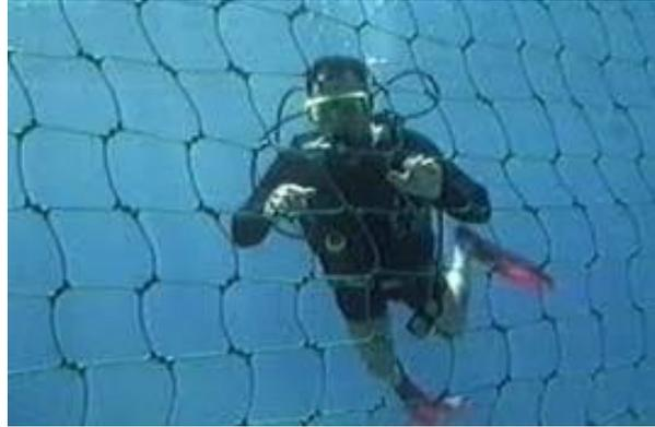
Spectron researched and developed the landmark for the perimeter security solution based on the fiber optic technology of detection principle. The system is designed to withstand all outdoor elements, from extreme freezing cold to deep ocean bottom depth. The UWMesh PIDS can be implemented in two manners which are,
